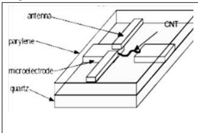
Fig.16: Schematic structure based on a nanoscale antenna of CNT [45].
