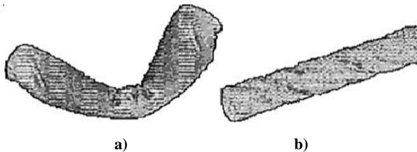
**Fig.2: The optimized bent tube a) at bending angle b) without bending angle [8].**
