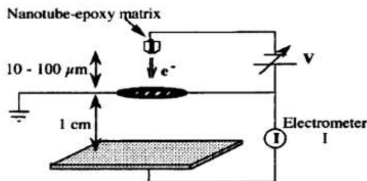
**Fig.12. Schematic of the carbon nanotube field emission with emission current transmitted detected by electrometer through the acceleration grid [36].**
