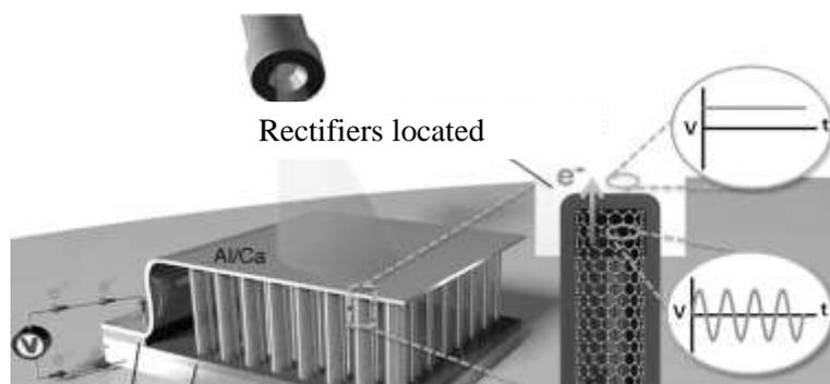
Fig.18: The scheme rectenna (rectifying antenna) as multi-layered carbon nanotubes and rectifier diodes [47].
