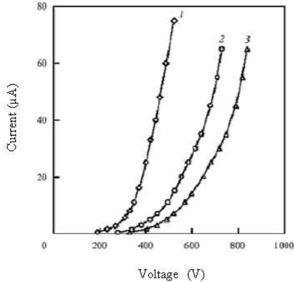
**Fig.3: The current-voltage characteristics of emitters with different orientations [13].**
