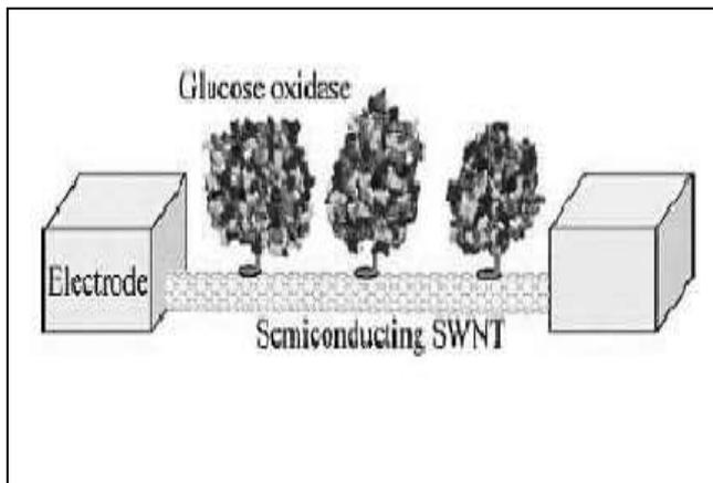
**Fig. 14: The biosensor on an individual single-layer carbon nanotube [38].**
