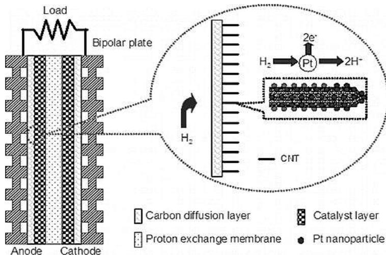
**Fig.13: The multi-walled carbon nanotubes used as platinum support for proton exchange membrane fuel cells have been investigated as increased utilization of platinum a way to reduce the cost of fuel cells [37].**
