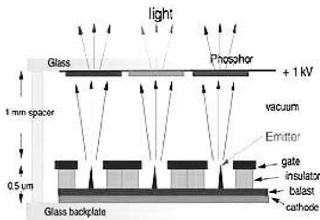
Fig.9. Diagram of the display based on CNT [31].
