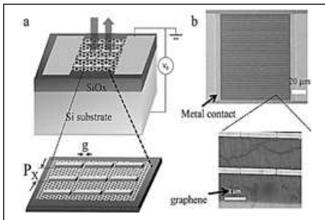
Fig.17: Array of nano-antennas a) An Si substrate b) A graphene and metal contains.
